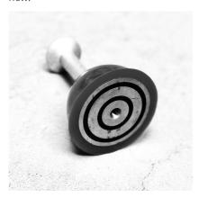
The recess former consists of a body of polyurethane in which a magnetic ring in a steel casing has been embedded. This improved design, has greater durability and magnetic force and is compatible with the P-anchors in load classes 13 to 100 kN.
